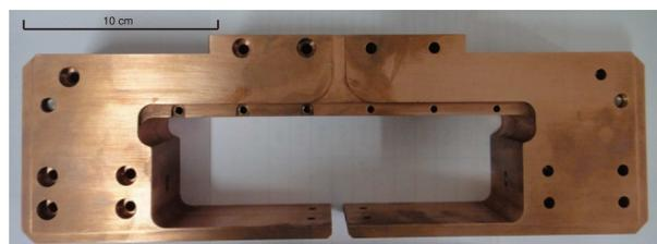
**Fig. 4.** (color online) The fabricated U-shape cavity.
