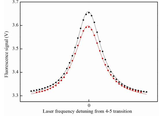
Fig. 2. The atomic beam spectrum versus the laser frequency near ( $F = 4 \leftrightarrow F' = 5$ ) transition. Black and red points are experimental results with microwave on and off respectively. The lines are fitted Lorentz lineshapes.
