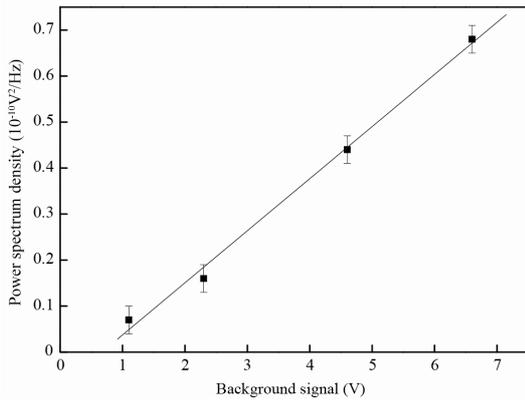
Fig. 3. The experimental data and fitted linear line of power spectrum density depending on the background signal with laser locked to the crossover line.
