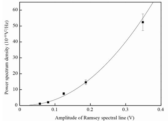
Fig. 4. The experimental data and fitted quadratic line of power spectrum density depending on the Ramsey line amplitude,  $U_s$ , with laser locked on the cyclic transition.
