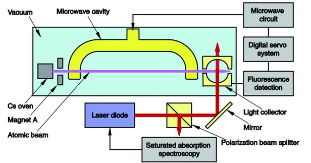
Fig. 1. Schematic diagram of our cesium beam clock.
