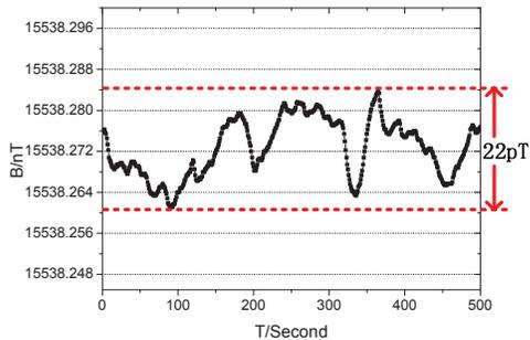
Fig. 5: 500 seconds long recording of a constant magnetic field with the NI PCI-4461 based digital-locking Cs magnetometer operated with the frequency switching method.
