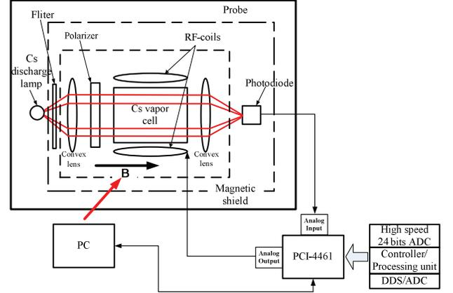
Fig. 4: Schematic diagram of the probe for detecting Zeeman transition signal and the digital servo system for locking the Zeeman transition frequency.
