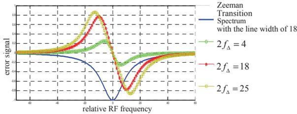
Fig. 3: Error signal (ES) curves under different frequency switching width (FSW).
