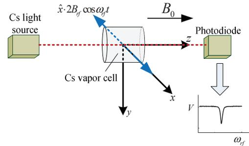
Fig. 1: Model of the probe for detecting Zeeman transition signal.
