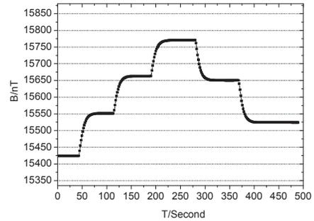
Fig.6: Recordings of the magnetometer's response to the change of the magnetic field.
