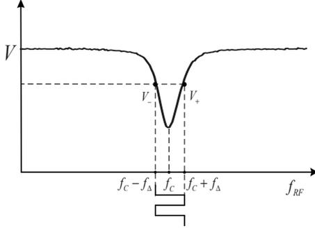
Fig. 2: Digital-locking method based on frequency switching between  $f_c - f_\Delta$  and  $f_c + f_\Delta$ .
