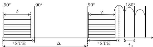
**Fig. 1.** The pulse sequence to measure D-T2 distribution functions with incremented gradient pulse amplitudes (rectangular area of width  $\delta$ ).
