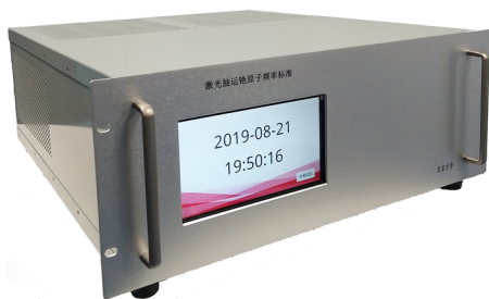
FIG. 15. The Peking University optically pumped cesium-beam frequency standard.
